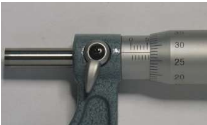
Metric micrometer's barrel and thimble
